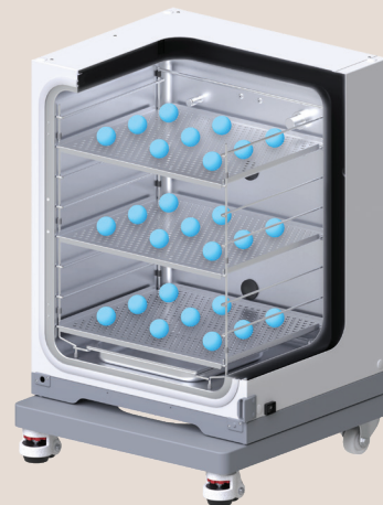
Fig. 1: Measurement set-up according to DIN 12880:2007-05 – 27 temperature probes placed at different locations on three shelves inside the CO 2 incubator
