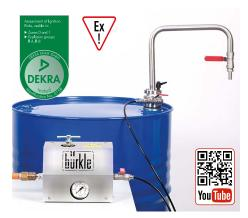
The withdrawal system can be used to dispense high-purity liquids quickly and without complications. An excess pressure is produced in the container with pressurised gas (compressed air or nitrogen), thereby pumping the liquid out of the tank. In this way, large amounts of hazardous media can also be safely dispensed and accurately metered. For use with media sensitive to oxygen or for ultra-pure media, operation with
